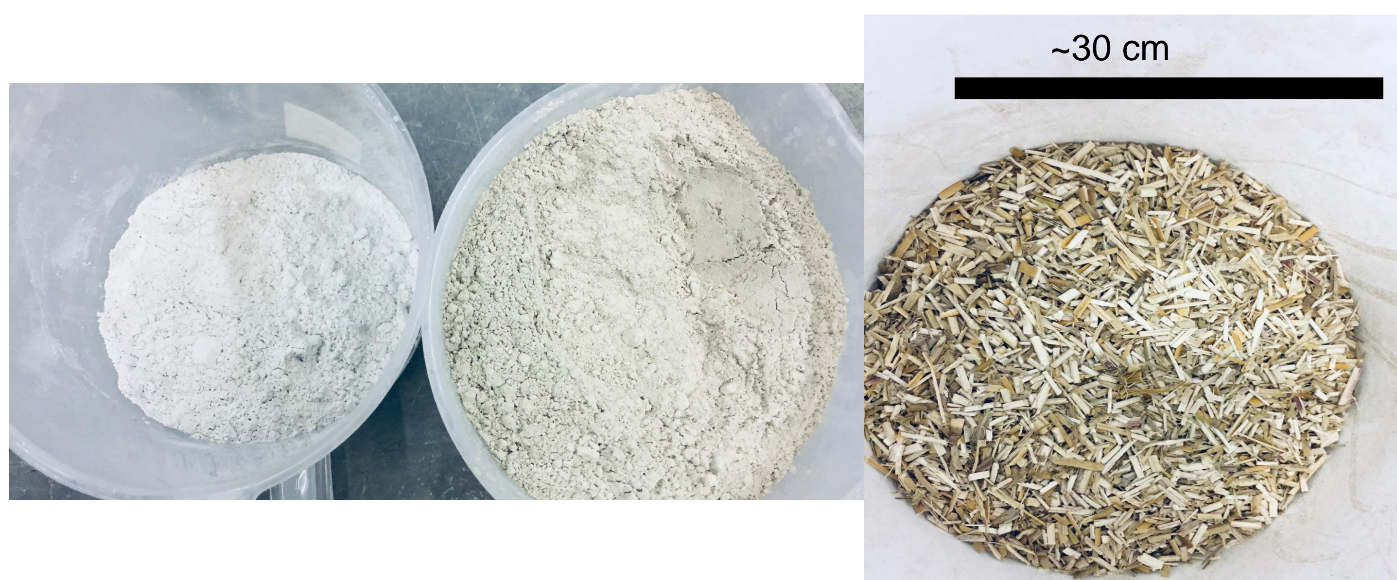
Fig. 1. Raw materials: hydrated lime, hydraulic lime and miscanthus particles.
