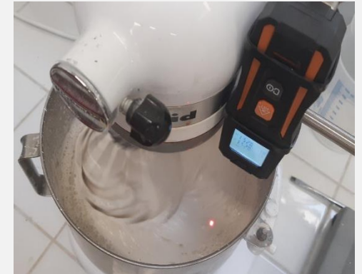
Direct foam method : Kitchen Aid mixer – bowl 5 l – 1 blade and 1 whisk
