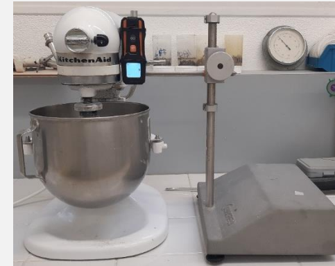
Direct foam method : Kitchen Aid mixer – bowl 5 l – 1 blade and 1 whisk
