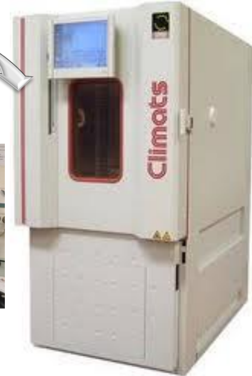
Climatic chamber EN ISO 12571 (2000)
